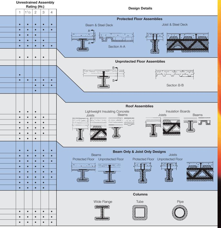
Note: Flutes above beams and joists must be filled unless otherwise allowed in the specific fire resistance design.
