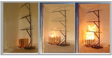
DESCRIPTION: Flame Seal-TB<sup>TM</sup> (aqueous based resin) is a spray applied fire protective intumescent coating, which satisfies thermal barrier / ignition barrier requirements of the IBC code when applied over Spray Polyurethane Foam (SPF) insulation.
