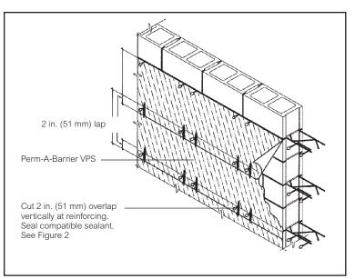
Figure 1: Membrane System Detail
