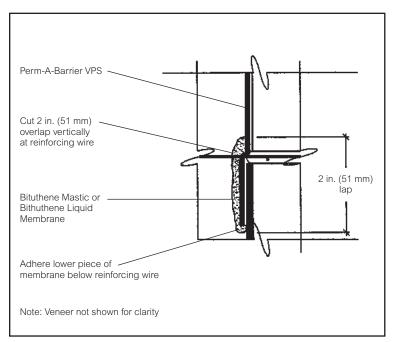
Figure 2: Horizontal Reinforcing
